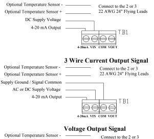
Optional Temperature Sensor + \_\_\_\_\_ 0-10 or 0-5 VDC Output Signal \_\_\_\_\_ Supply Ground / Signal Common \_\_\_\_\_\_ AC oe DC Supply Voltage \_\_\_\_\_
