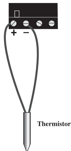
Wiring a Temperature Sensor
