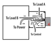
\* Isolate any unused wires, e.g. wire nut.
