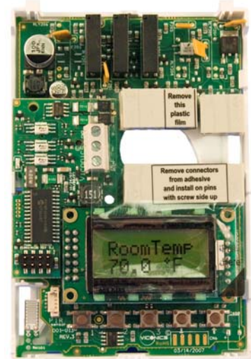
Thermostat assembly (VT7300F5000B shown)
