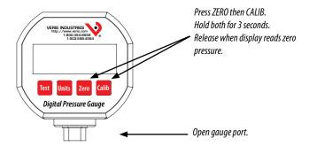
The PD can be re-zeroed without affecting the span calibration. The gauge port must be open with no pressure or vacuum applied.
