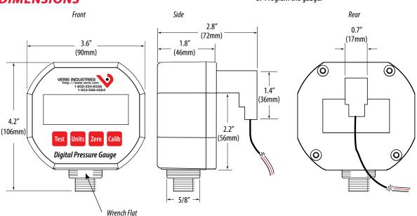
(Tighten with a 5/8" wrench at this spot. Do not tighten by twisting the plastic PD housing.
