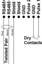
4. *Modbus Hookup:* Attach any Modbus slave or master devices to the RS-485 terminals as shown in the wiring diagram. Multiple Modbus devices may be attached to each H8830.
