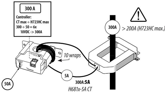
**! DANGER: 5A CTs can present hazardous voltages. Install CTs in accordance with manufacturer's instructions. Terminate the CT secondary before applying current.**
