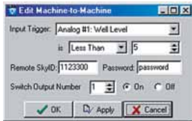
Figure 4: Turn Pump On if Level is Less than 5 feet
