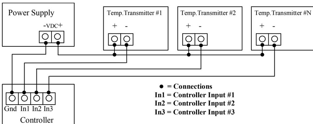
All ACI/TT and TTM temperature transmitters are reverse polarity protected.
