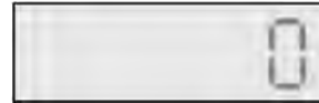
Fig. 2: Upon startup for the -EC models, counter should read zero. If a non-zero is displayed, the counter can be reset by following Step 6. If the counter is blank, contact MCG Support at 1-800-851-1508.
